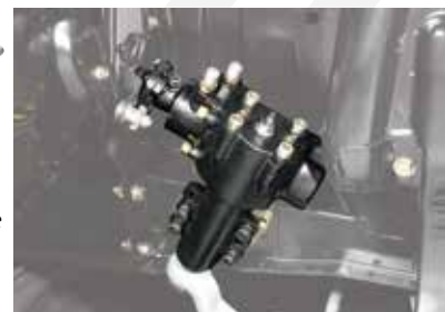
CPP's new 400 Series™ Power Steering Box is compact and lightweight but really packs a punch!
