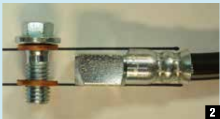
2. The reference marks indicate "top" and "bottom" of the banjo fitting; the stepped side (top) faces outward, allowing the bottom to seal tight onto the caliper without coming in contact with the fitting's crimped shoulder. (photo 2)
