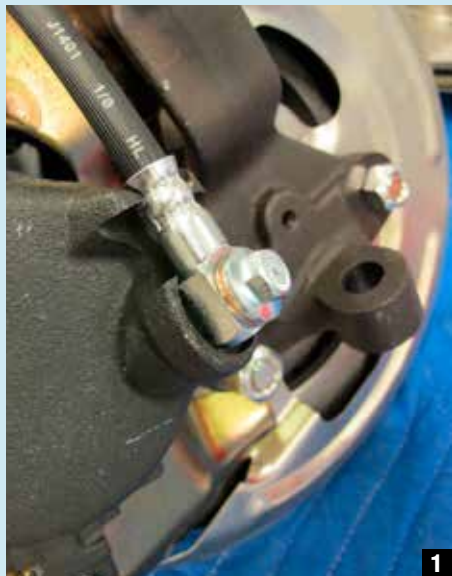
1. Banjo-style rubber brake hoses with an offset fitting must be installed with the notched side facing outward in order to attain a complete, proper seal. (photo 1)
