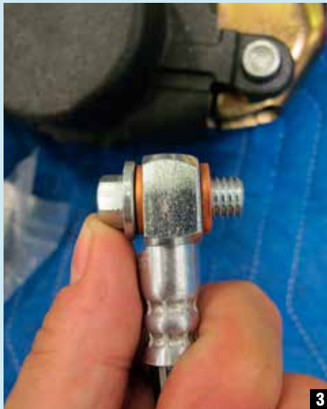
3. Always use copper compression washers on both sides of the banjo fitting. (photo 3)
