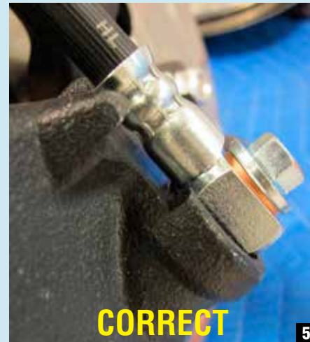
5. Properly installed and tightened, no portion of the brake hose fitting (other than the copper washer) should come in contact with the caliper body, as shown. (photo 5)
